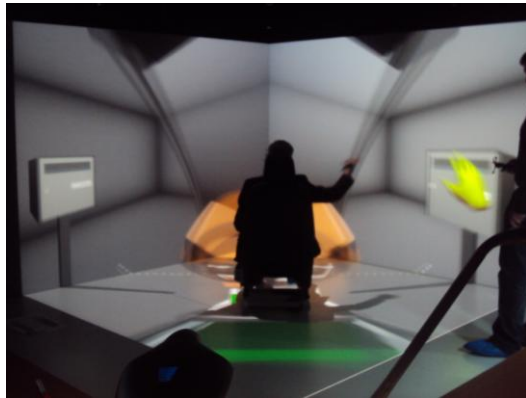
Fig. 7 The ergonomist took the place of the postman on the VR platform. He was trying to touch the right mailbox. The virtual hand changed its colour when the actor touched the mailbox.
