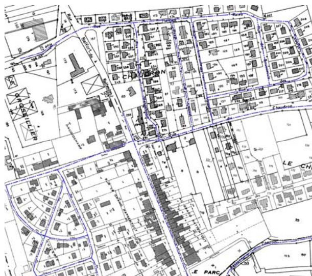
Fig. 7 Part of the plan of the main drinking water network in the town of "Dieu-sur-Mer" 14 -France- dated 2007.
