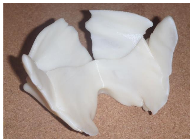
Fig. 13 Results of the 3D printing of the pelvic floor in ABS
