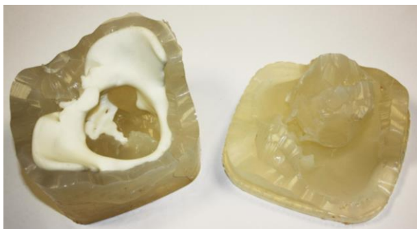
Fig. 14 Vacuum casting of the prototype of pelvic bones in PU
