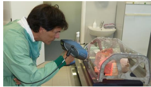
Fig. 2 Scanning device with RevScan (CREAFORM)
