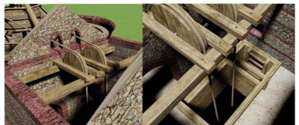
Fig. 15 Detail of rendering of pulleys and well
