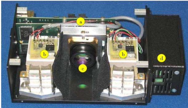
**Fig. 2 3D-CMOS sensory system. Which is composed by the electronics board including the array sensor chip (a), laser illumination modules (b), image optics (c) and power supply (d).**
