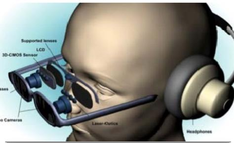
**Fig. 3 Integration of the environment scanning elements: the laser illumination modules and the image optics into a pair of glasses.**
