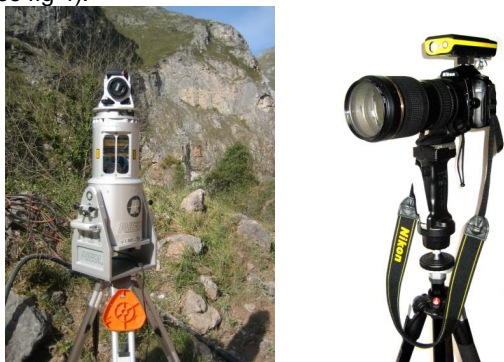
Fig. 4 RIEGL LMS-Z390i scanner and the calibrated camera Nikon D90
