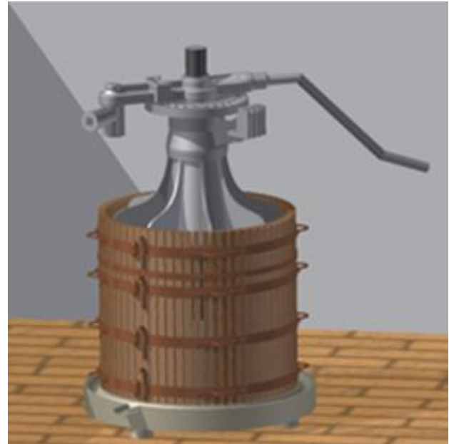
Fig.5. Vertical Samain press of double speed
