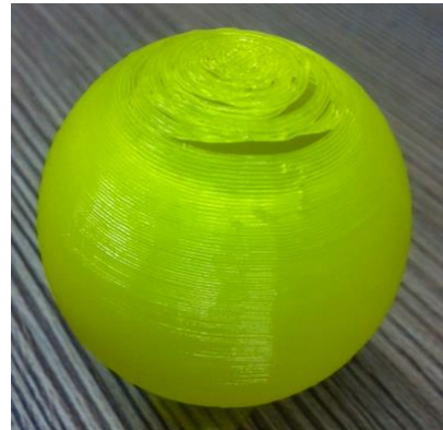
Fig. 6 aberration in slicing volume with thin surface
