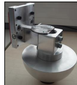
Fig. 4 Impact testing support assembly
