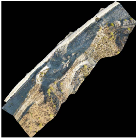
Fig. 9 Orthoimage of the embankment obtained from the vertical photogrammetric project.
